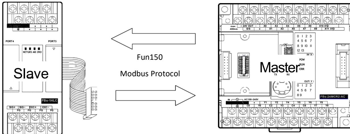
Connect to PLC using Winproladder and change the PORT 3 communication parameters of Winproladder. The communication parameters of 1HLC are fixed as follow:
