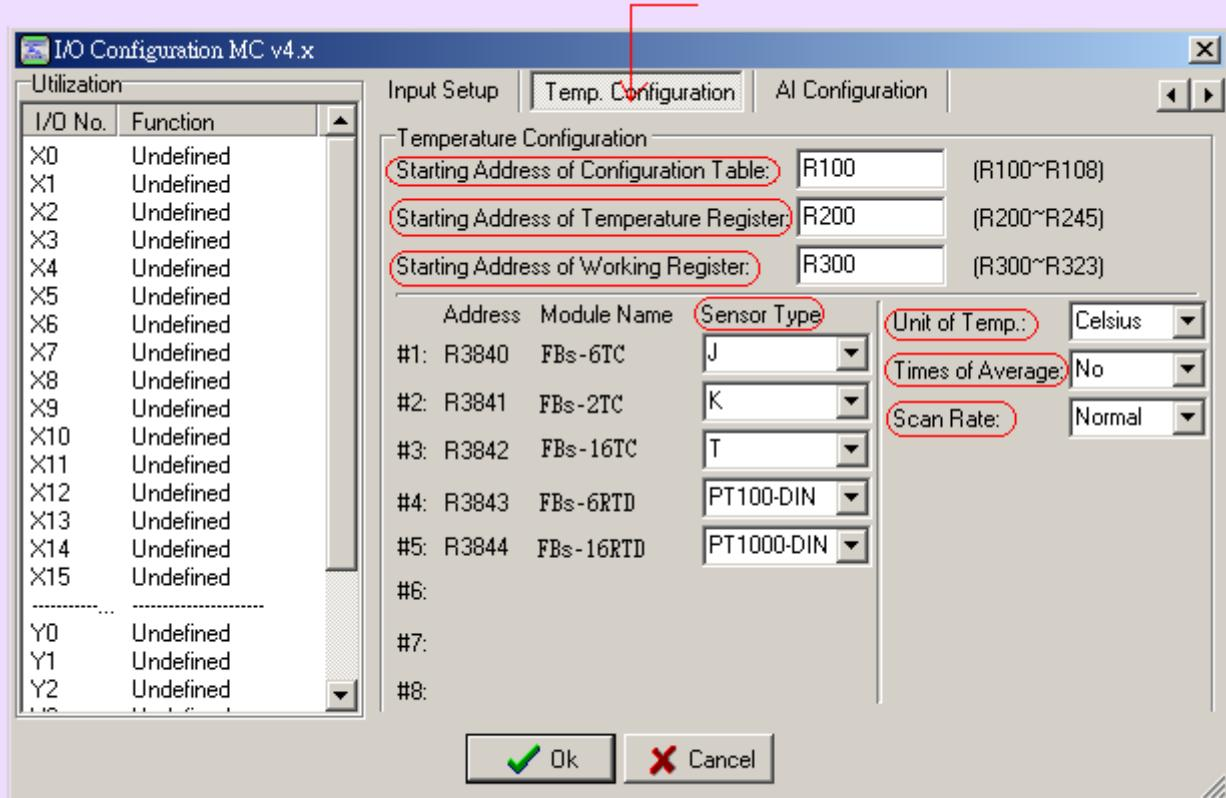
The user need to assign a starting register of a contiguous register area for holding temperature reading value and areas for storing the configuration table and working scratchpad and define the sensor type, unit of temperature, scan speed and samples for average. Please refer the advanced manual II for detail explanation.
