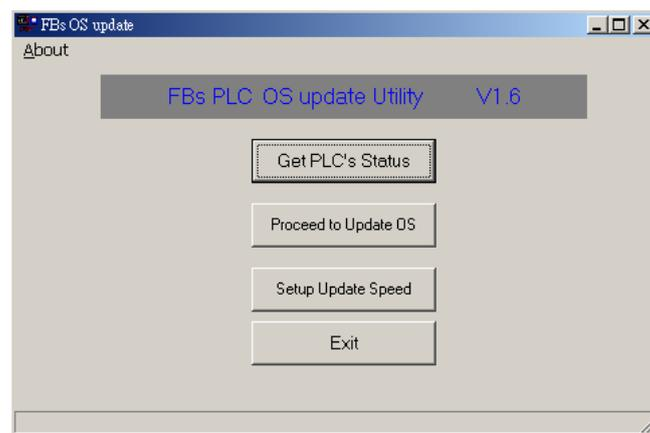
To speed up the whole OS update process, the program download speed can be set differ than the current connected speed. Click the [Setup Update Speed] button to popup the following screen.
