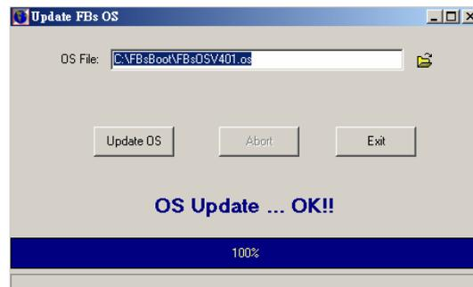
Should the update process is fail in half way due to the power failure or other reasons, the PLC will stay in update state which can recognize by watch the 'long-short-short' flash pattern of 'RUN' LED. Under such circumstance should repeat the step 7 ~ step 8 operation.
